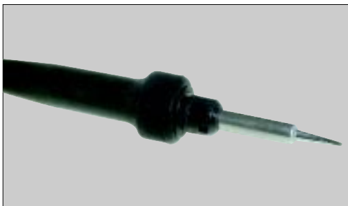
Soldering iron with precision ceramic heater
